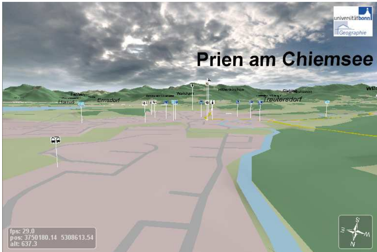
Figure 1: examples of OSM road and land use data that has been combined with a SRTM 3 arc-seconds (ca. 90m) terrain model. Primary and secondary roads have been flattened more than cycle ways and little forest tracks. Thus a more natural appearance is achieved.
