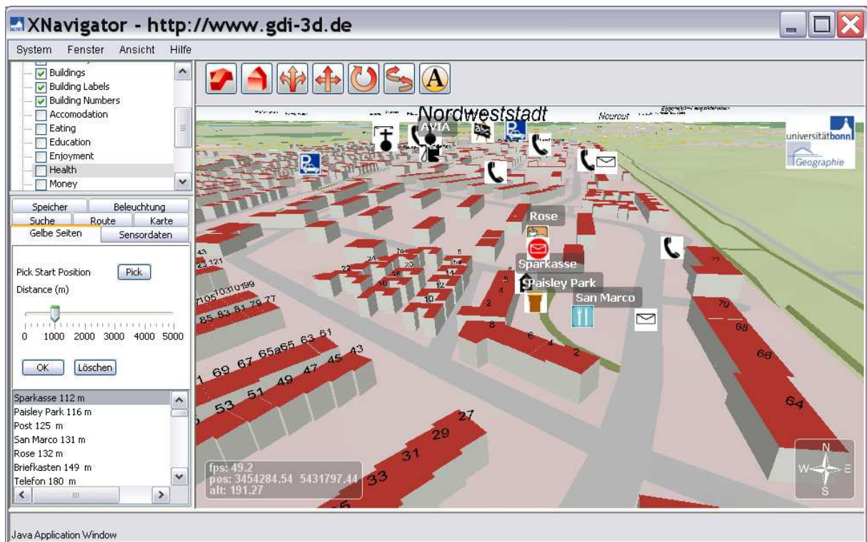
Figure 2: Web based 3D service based on combining OSM and SRTM: buildings extruded into 3D and POIs displayed as 3D symbols delivered from OpenLS Directory Service. Presented is the city of Karlsruhe based on OpenStreetMap data combined with SRTM data.
