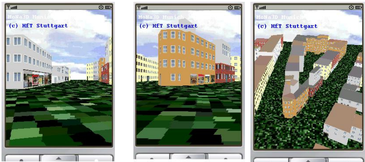
Fig 1: Prototype implementation: 3D city model of Munich on mobile device using tile based textures. © HFT Stuttgart, data provided by Tele Atlas
